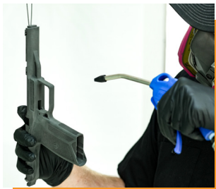
Before spraying, blow off all parts.
