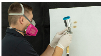
Testing spray gun settings before application.
