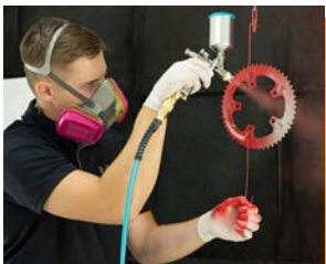
When spraying, part should appear wet.
