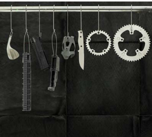
Metal hooks are ideal for racking larger parts.
