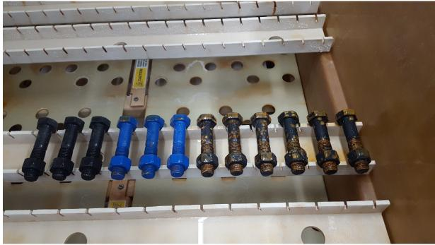
Photo 1. All four coatings in salt fog chamber at 24 hours.
