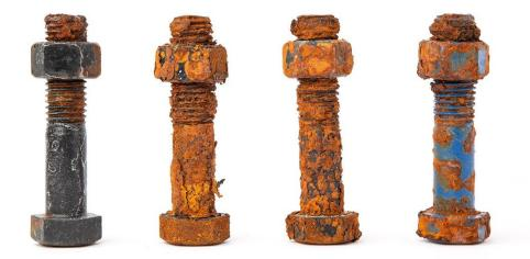
**Photo 12.** Corrosion levels of Cerakote Blackout after 4,000 hours, Teflon Black and Teflon Metallic Black after 640 hours, and Xylan after 1871 hours.
