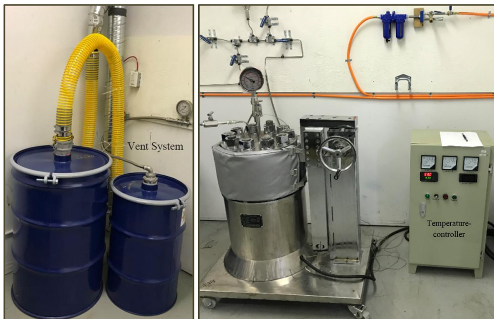
Figure 2. Example of the Autoclave Test Setup
