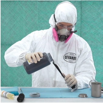
1.) Pour the desired quantity of Cerakote into a glass graduated cylinder (SE-147A).
