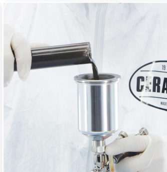
4.) Pour mixed coating through a 150 mesh strainer for most* H-Series products, as shown (NIC Part # SE-276).
