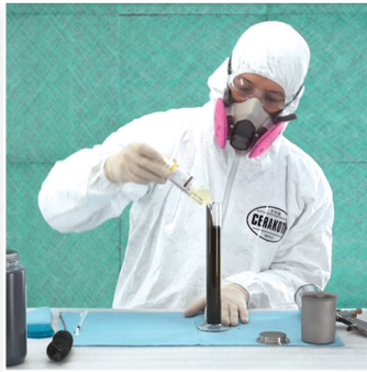
2.) Add the catalyst. Use table 1 pg. 11 to determine Cerakote to catalyst ratio for finish type.
